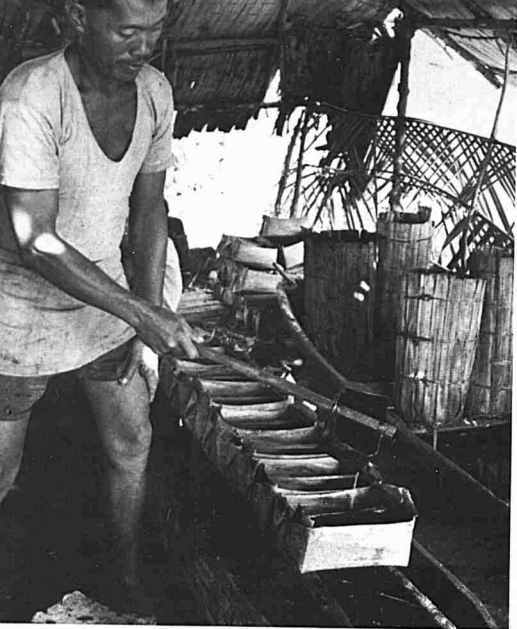
Paloh, in the delta of the Rejang, has a long tradition of salt making. The roots and stems of nipa palms which have floated down to the sea are burned and the ashes, which contain a high proportion of salt, are collected. Sea water is poured through the ashes and the salt is washed out to produce a saturated solution for boiling down in oblong, bark containers. The latter can be used only once and must then be thrown away.
