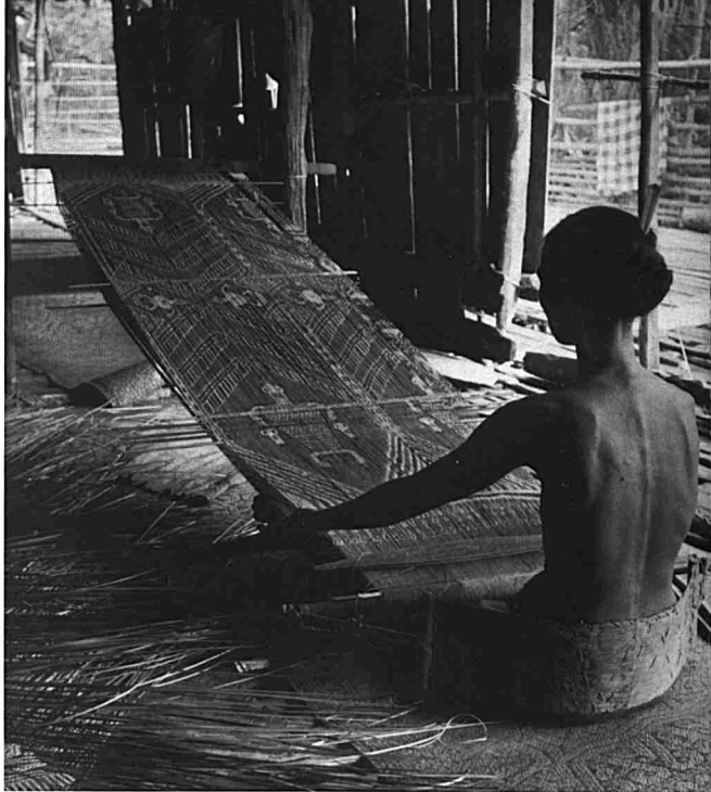
Weaving a blanket (pua kumbu). The loom is a simple but effective one. The woman leans back against the bark cloth girdle to brace it taut as she moves the shuttle to and fro. Such blankets are made for ornamental purposes. They adorn the longhouse walls during parties and are used to cover mattresses provided as seats of honour for guests but for the rest of the time they are put away in chests.
