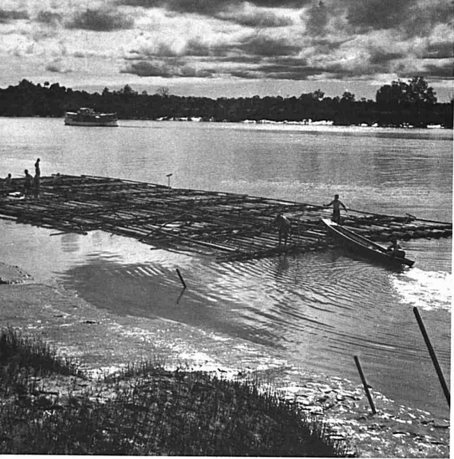
A log raft near Linga in the 2nd Division ready to be towed out to an ocean-going ship for loading. Such rafts must be stoutly made to stand up to the strong tides and currents which are a feature of the rivers near their mouths. Another source of difficulty are the bars at the river mouths which generally hinder the approach of shipping. Only at the mouth of the Rejang can large ships cross the bar.
