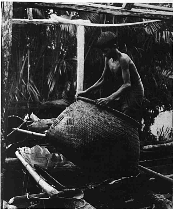
The rasped pith is placed on a mat or in a large basket and stamped on and shaken while water is poured over it. The basket technique is used in the Matu area of the 3rd Division, while in the Mukah and Oya Rivers mats are favoured. The water washes out the sago which settles as a white cheesy mass in a trough below. After it has been dried it is ready for export.
