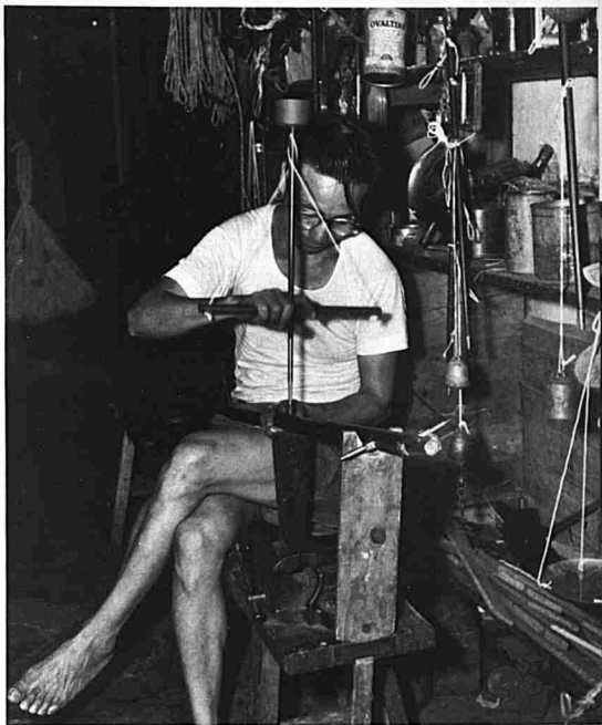
Chinese scales or daching are universally used throughout the country and are made by craftsmen in Kuching. The mode of manufacture and especially the drill are typically Chinese. It is remarkable how Chinese crafts are maintained abroad even by those Chinese who have never set foot in the land of their ancestors.
